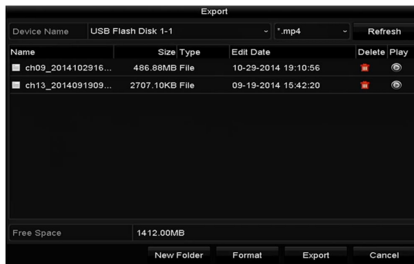
Figure 9-2 Quick Export using USB1-1
