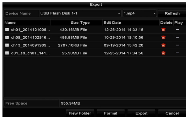
Figure 9-6 Export by Normal Video Search using USB Flash Drive
