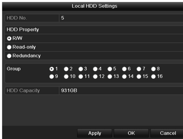
Figure 13-5 Local HDD Settings
