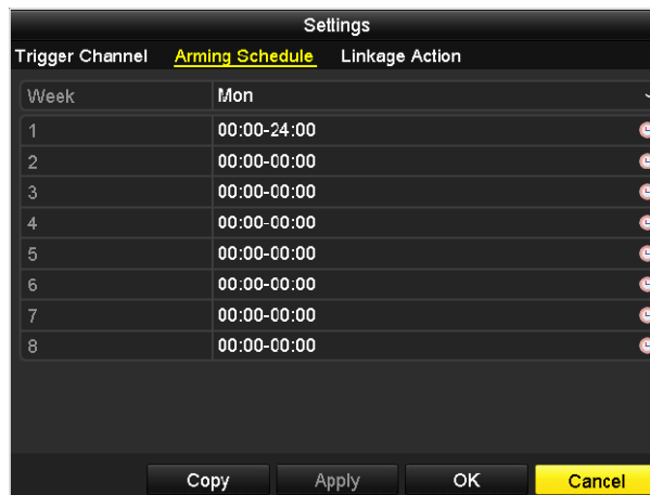
Figure 10-3 Set Arming Schedule of Motion Detection
