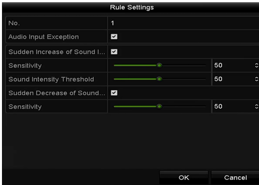
Figure 10-22 Set Audio Exception Detection Rules
